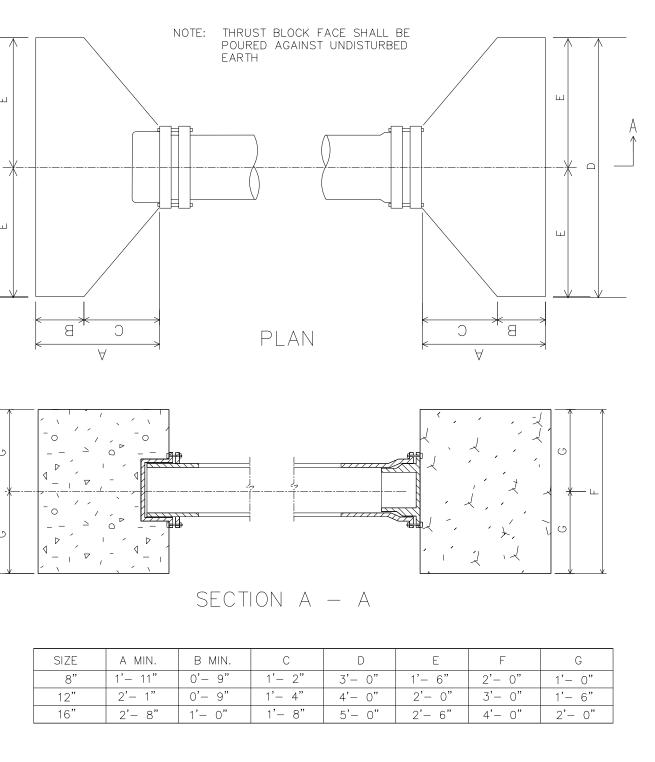
CONCRETE THRUST BLOCK FOR ENDS
